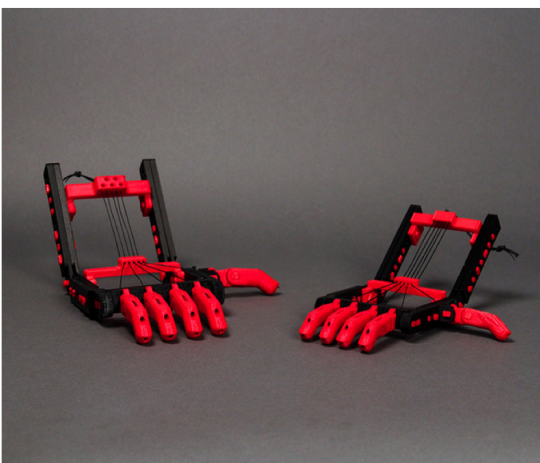
Robohand, an open-source robotic hand that can be downloaded and adapted. Source: Robohand on Thingiverse.
