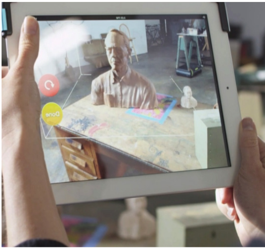
Demonstration of the 3D Structure Sensor scanner connected to an iPad. Source: Occipital.
